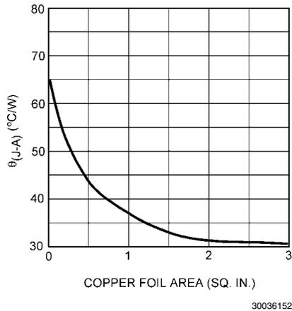
FIGURE 5.  $\theta_{JA}$  vs Copper Area for TO-263 Package
